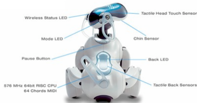
Figure 50: AIBO Features - Back [Source: Sony AIBO-Europe Homepage]
