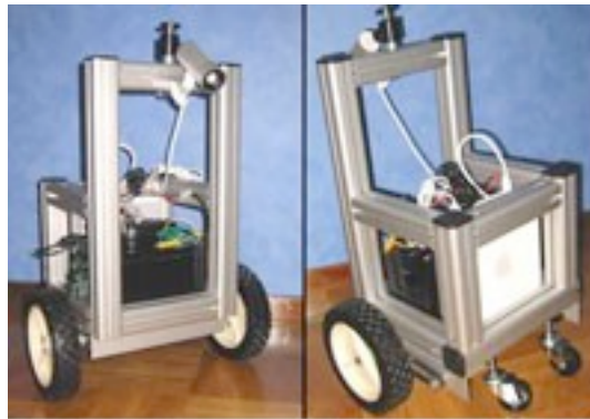
Figure 29 The MiniBot, a prototype mobile robot which will be used to move the camera while it is tracking dynamic scenes like the fish game and marble game.
